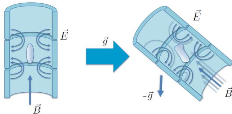
**Figure 1.** Left: The electron is trapped in an ideal Penning trap consisting of an electric quadrupole field and a constant magnetic field. Right: The presence of a gravitational field changes the dynamics of the trapped electron and the properties of the electromagnetic trapping field.
