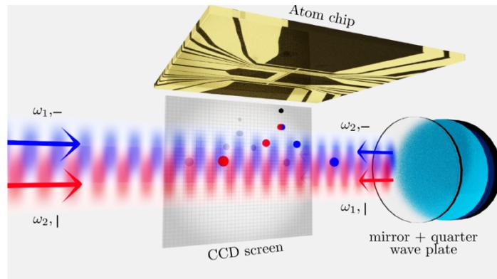
**Figure 1.** Scheme of the twin lattice generated by a light field of two frequency components retro-reflected of a mirror surface to drive symmetric double Bragg diffraction and Bloch oscillations.
