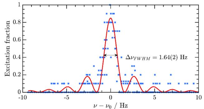
**Figure 1.** (left) Image of the new ion trap, under construction. The flange diameter is 40 mm. (right) Quantum excitation fraction of the E3 transition driven with 500 ms pulses, Fourier-limited to 1.6 Hz.
