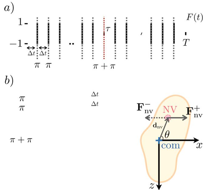
**Figure 1.** Summary of the setup. (a) Sequence of pulses acting on the NV center. (b) Schematics of the paths of the interferometer. (c) Irregular nanodiamond hosting an NV center and the forces acting on it.
