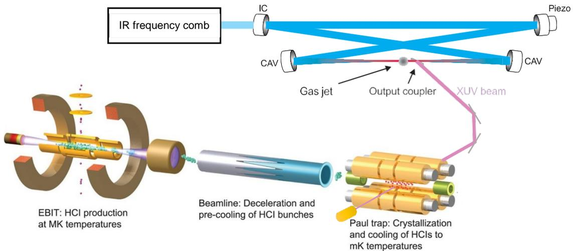
**Figure 1.** Scheme of an experiment combining a VUV frequency comb based on high-harmonic generation within an enhancement cavity with a RF trap for highly charged ions.
